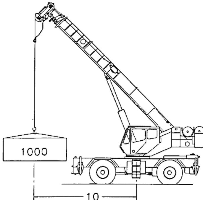
If we increase the radius such that this load acts upon a twenty unit radius, the load moment has increased to twenty thousand units
