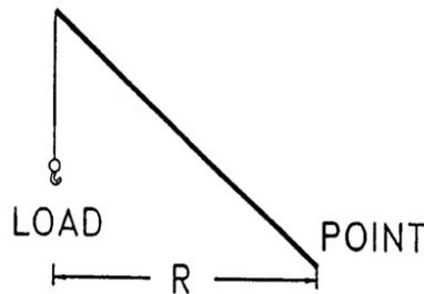
In the case of cranes, the force acts vertically through the center of gravity of the load and the moment arm becomes the horizontal distance from this center of gravity of the load and the center of rotation of the crane. Therefore, with a one thousand unit force acting at a ten unit radius the load moment is the product of these two factors or ten thousand units as shown below.
