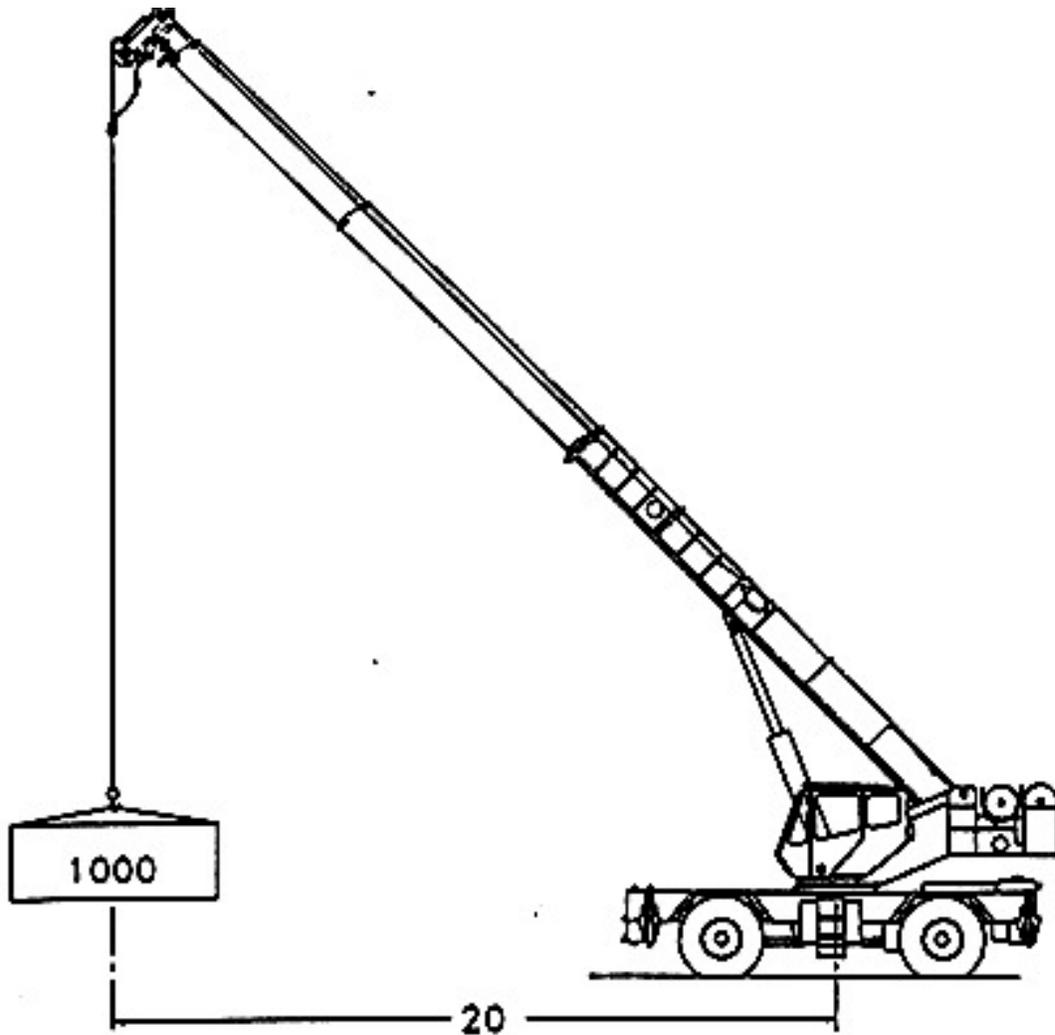
In this example the load on the load line has remained the same but the load on the crane, the load moment, has actually increased by a factor of two. Because load moment is used to determine the capacity of a crane, crane load charts require the operator to determine not only the magnitude of the load but the radius that the load is acting upon. Since load moment is a product of these two each value becomes equally important.
