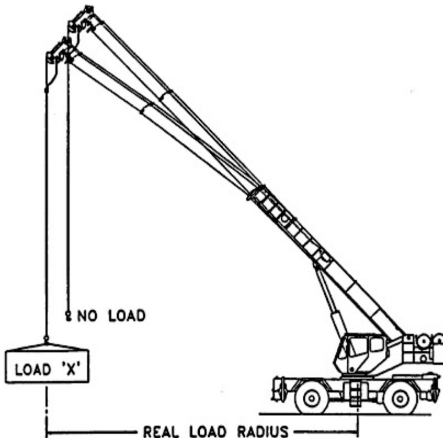
This increases the load moment proportionately. An increase in radius of 15% has increased the load on the crane by 15%. It is extremely important that the operator be aware of these dynamic changes effecting the crane.
